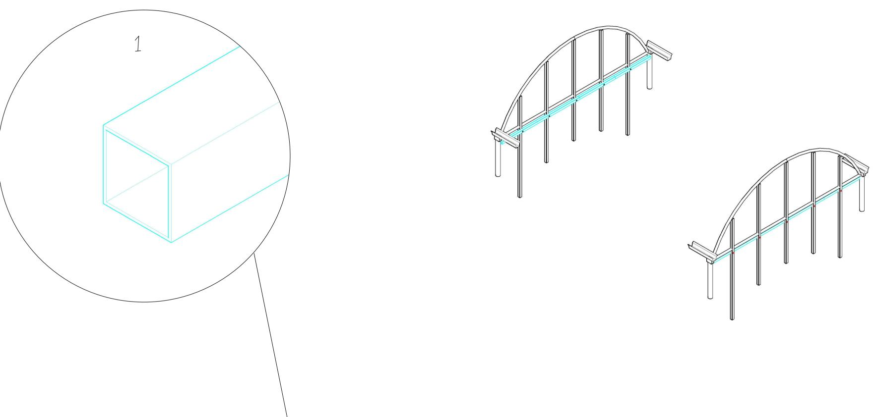
WHEN POSSIBLE MOUNT THE TUBING ON THE OUTER SIDE OF THE GABLE STRUCTURE. THIS TO PREVENT THE POSSIBLE NEED OF A SLIP SECTION IN THE LAST BAY OF THE SYSTEM.
