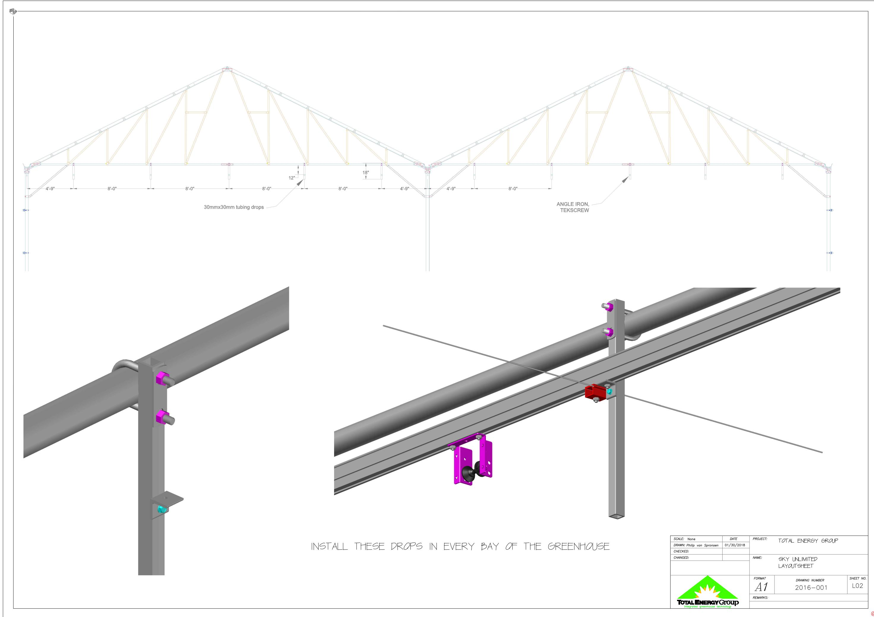
BEGIN INSTALLATION OF SYSTEM BY INSTALLING SUPPORT TUBING AT BOTH ENDS OF THE GREENHOUSE AS SHOWN IN ILLUSTRATIONS. KEEP IN MIND THAT THERE HAS TO BE A CLEAN LINE OF SIGHT FROM ONE END OF THE GREENHOUSE TO THE OTHER END TO LET THE SYSTEM TRAVEL FREELY. THE LAYOUT OF THIS TUBING WILL DETERMINE THE SHAPE OF THE SHAPE SYSTEM.
